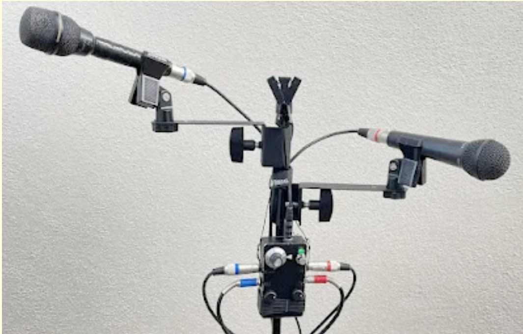
The Mixer/Preamp and the mics. Balance, Volume, Clipping detection, and Mute are all controlled from the mic position
